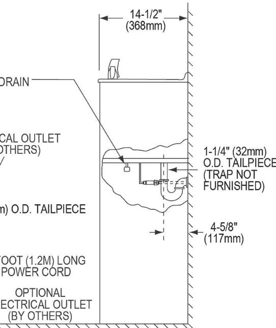
NOTE: INSURE PROPER VENTILATION BY MAINTAINING 4" (102mm) MINIMUM CLEARANCE FROM CABINET LOUVERS TO WALL ON EACH SIDE OF COOLER.
