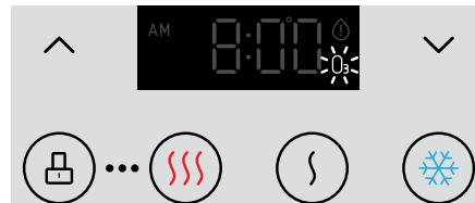
During the cleaning cycle, ozone is produced and injected into the water system. This ozone kills bacteria and biofilms typically found in water dispensers. By the time the cleaning cycle ends, the ozone is converted to harmless oxygen and emitted into the air.
